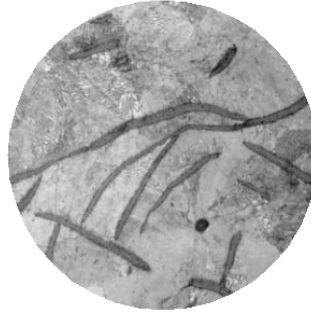
Photomicrograph Showing Graphite Form in Gray Iron
